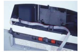
This assures that the imprinter cable will not be pulled too tightly when the scanner door is opened.
